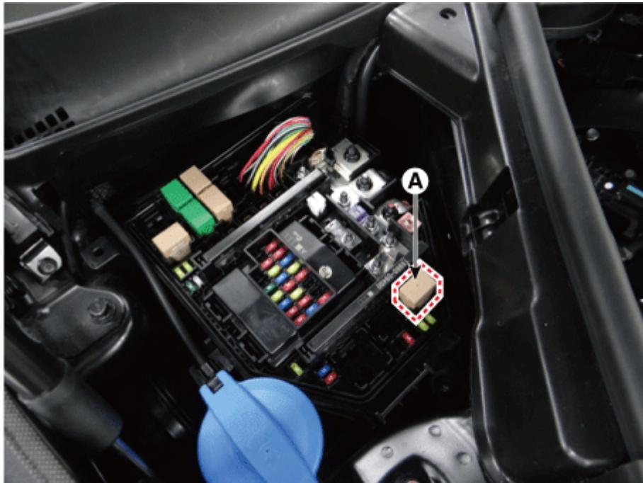
4. Check for continuity between the terminals (30 and 87) using an ohmmeter.
